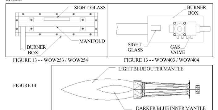
There is no primary air adjustment on the burner and with correct installation, a proper flame is assured; since the correct manifold pressure and orificing has been done at the factory for elevations up to 2,000 ft.
